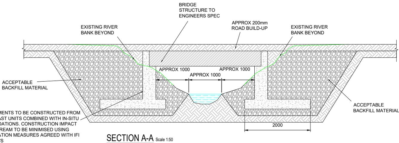
ABUTMENTS TO BE CONSTRUCTED FROM PRECAST UNITS COMBINED WITH IN-SITU FOUNDATIONS. CONSTRUCTION IMPACT ON STREAM TO BE MINIMISED USING MITIGATION MEASURES AGREED WITH IFI & NPWS
