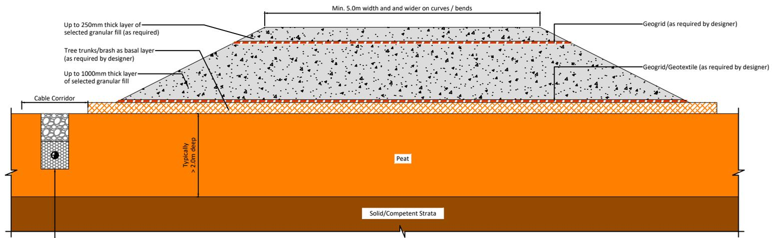
Indicative cable duct trench (only located on one side of roadway across majority of the site). Cable trench can be located on either side of the road surface but where possible it should be located on the upstream side of the road surface.
